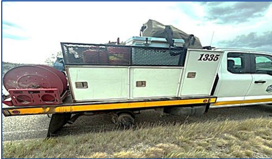
The engine after the passenger-side outer dual tire “exploded” and the inner dual tire rolled off.
